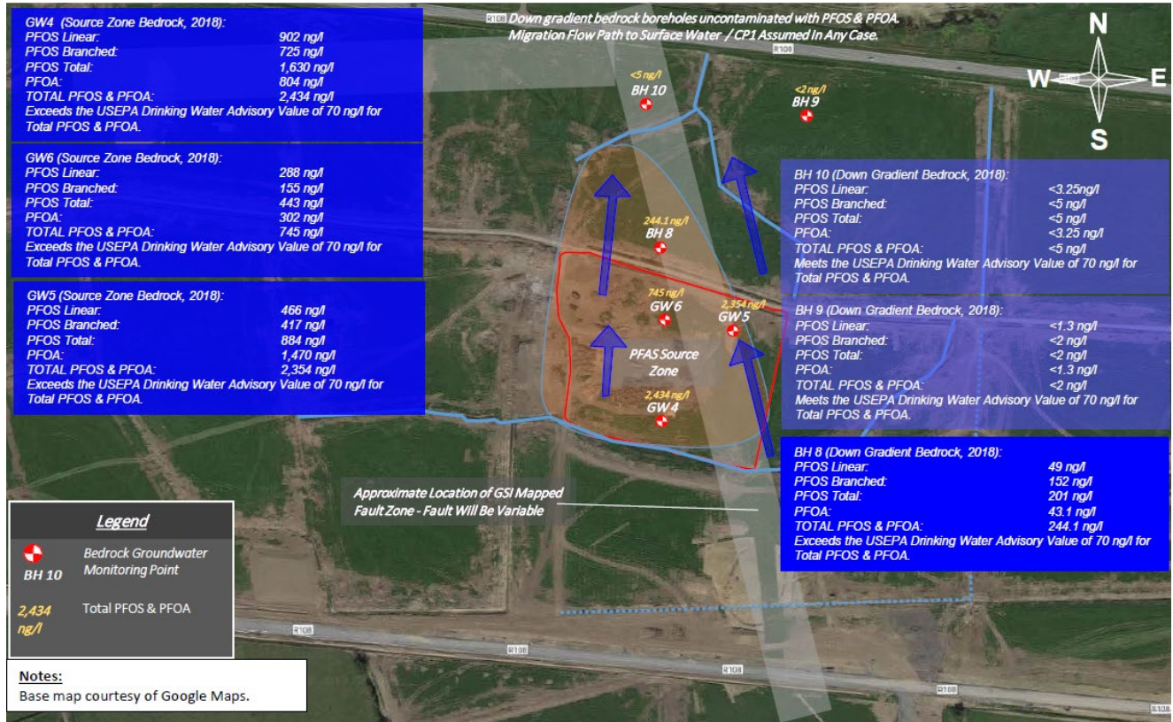
Figure 3-3: PFOS and PFOA Sample Results from Shallow Borehole Bedrock Samples 2 prepared by IE Consulting and Reproduced from the May 2018 DQRA
