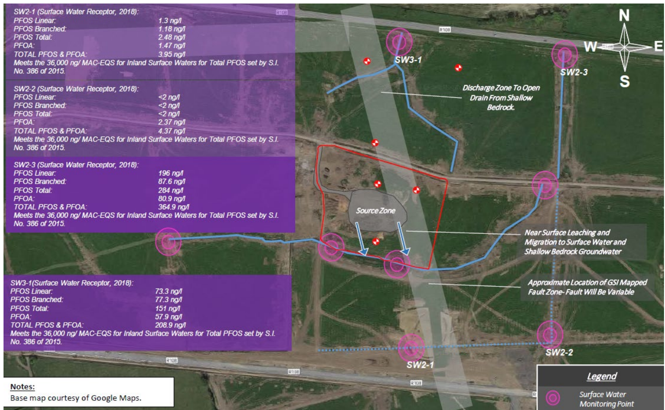
Figure 3-4: PFOS and PFOA Sample Results from Surface Drains adjacent to APEC 5 2 prepared by IE Consulting and Reproduced from the May 2018 DQRA
