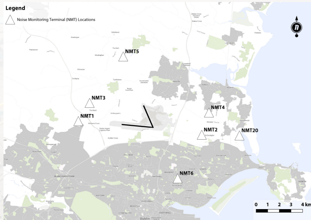
Figure 2: Noise Monitoring Terminal locations
